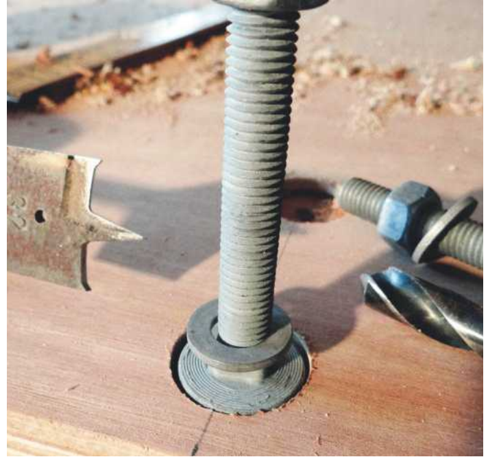
▲ Pic.10 Once the hole is bored for the bolt, it's too late to use a flat bit for the necessary countersinking because it has nowhere to centre itself. Use the flat bit first and then drill the bolt hole
